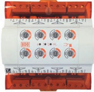
Available in both analogue and digital variants, Trend's new IQ®4 Hand/Off/Auto (HOA) modules make it possible to override plant when a controller/strategy is not achieving the results required. These devices also enable plant to be overridden for testing and can be used for commissioning, as they work straight out of the
