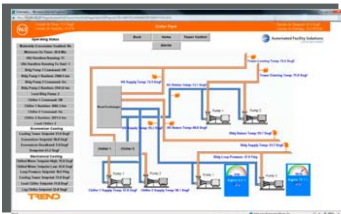
A Quintiles Plaza chiller plant: Trend's 963 Supervisor front-end software gives building staff quick, comprehensive views of the entire system.
